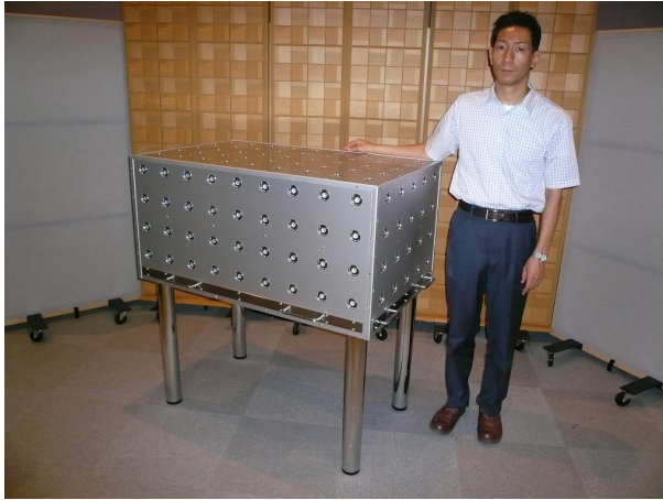
Fig. 5 Image of radiated loudspeaker array
