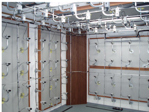
Fig. 2 Near 3D sound field reproduction system using directional loudspeakers and wave field synthesis [8]
