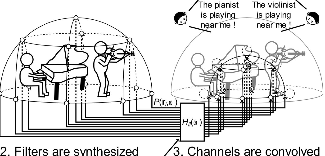
2. Filters are synthesized from acoustic transfer functions  $D_{s}(\mathbf{r}',|\mathbf{r}_{i})G(\mathbf{r}',|\mathbf{r}_{i},\omega) \triangle S'_{i}$
