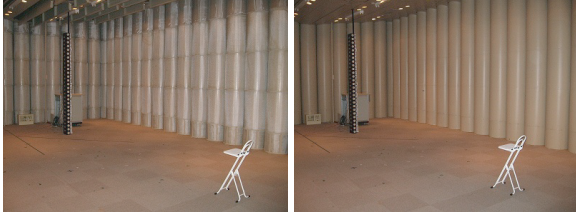
Fig. 3 Image of experimental environment in the listening test (Left: Reverberation time 140 ms, Right: Reverberation time 1030 ms).
